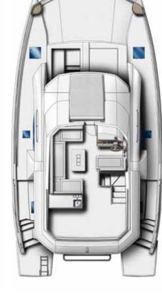
The Leopard 43 Powercat is available in either a 3 cabin, 3 head version, or a 4 cabin, 4 head version. Both layouts offer the option of additional storage, berth, or head in the forward hull.
